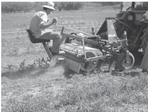
Figure 5. Horizontal brush weeder at work. Back steering allows high crop selectivity.
