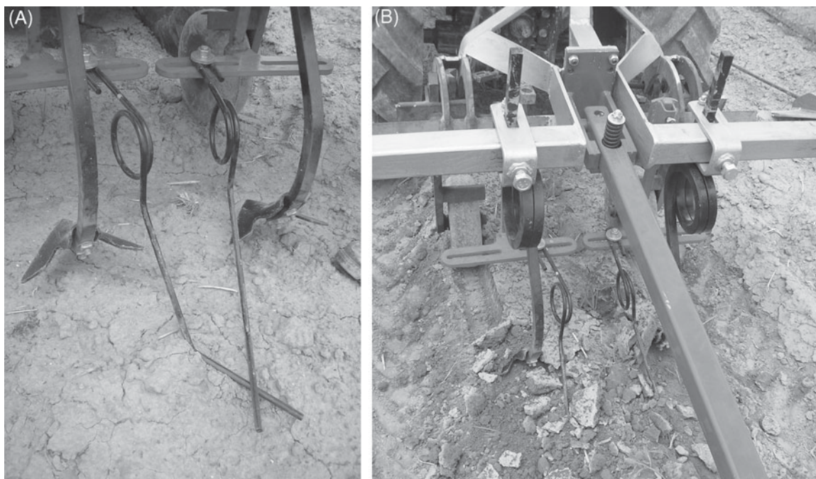
Figure 3. Torsion weeder (center) and cultivation blades at the sides. The tips of the torsion weeder work in the soil at an approximate depth of 3 cm.
